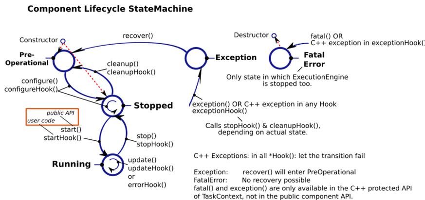
This figure shows the extended state diagram of a TaskContext. This is Figure 2.5, “TaskContext State Diagram ” extended with two more states: Exception and FatalError.
