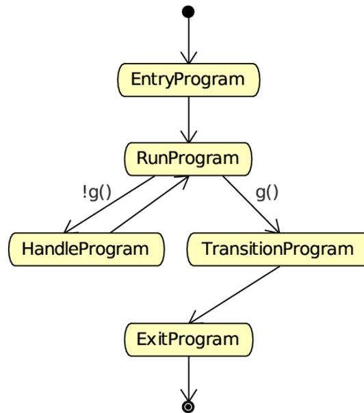
The automatic mode additionally actively evaluates guard conditions. Event reaction remains in effect, but is not shown in this diagram.
