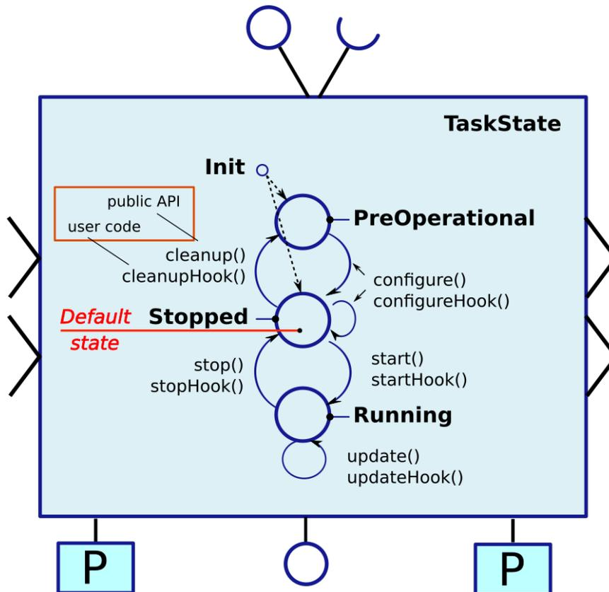
During creation, a component is in the Init state. When constructed, it enters the PreOperational or Stopped (default) state. If it enters the PreOperational state after construction, it requires an additional configure() call before it can be start()'ed. The figure shows that for each API function, a user 'hook' is available.
