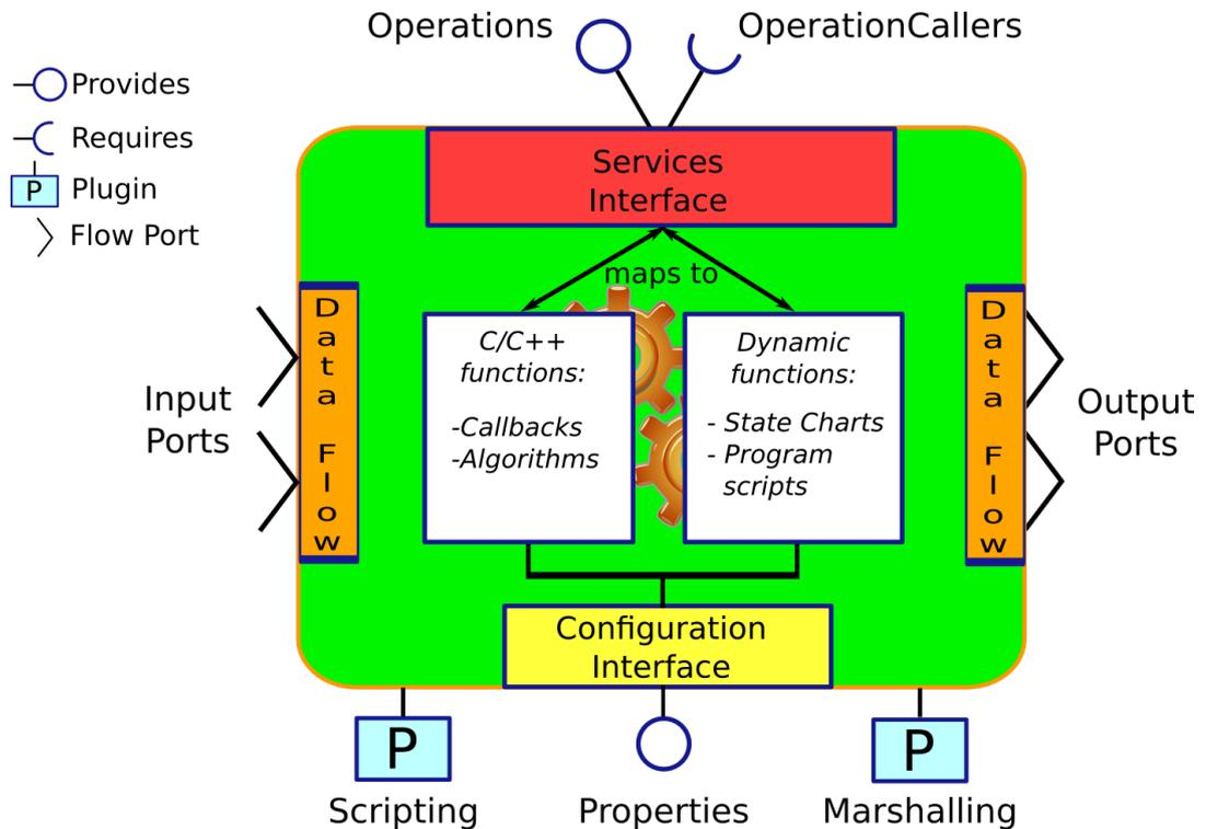
The component offers services through operations, and requests them through operation callers. The Data Flow is the propagation of data from one task to another, where one producer can have multiple consumers and the other way around.
