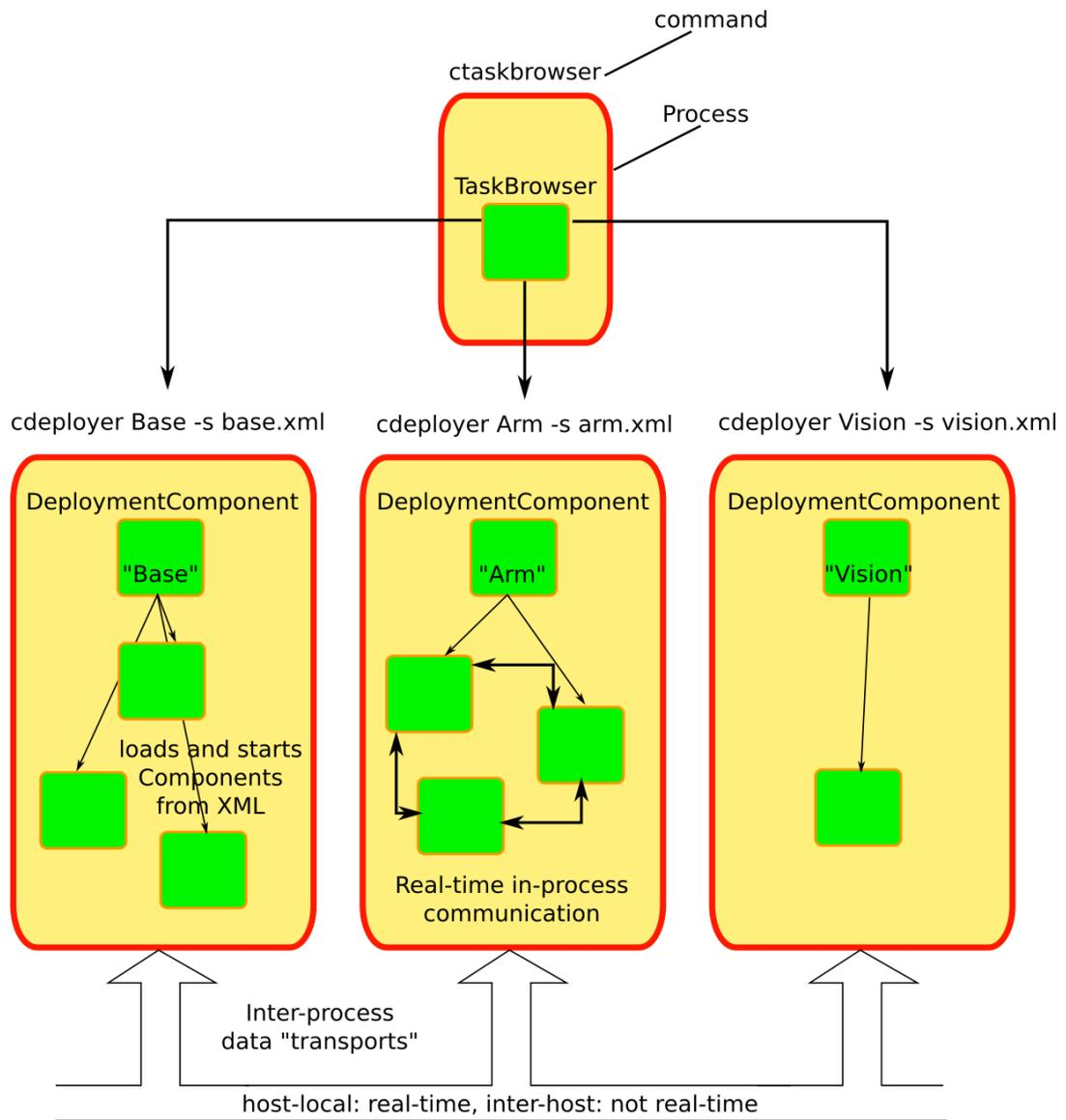
Components are loaded into the process by a deployer, which gets its configuration through an XML file. Communication between processes is transparent to the component, but your data must be known to Orocos (cfr 'typekits' and 'transports'). Most new users start with a single process however, using the 'deployer' application.
